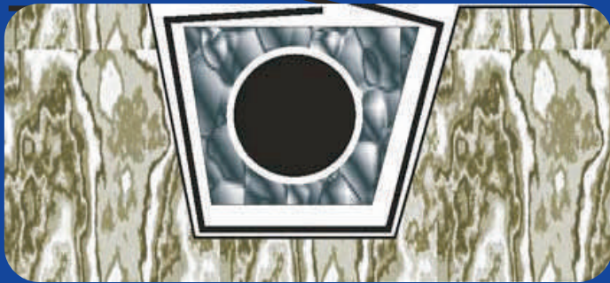
Diagram showing Geocil Filterfab used in a wrapped drain
